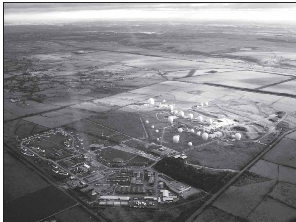
A birds-eye view of the Menwith Hill Royal Air Force Base in the Yorkshire Dales, the largest electronic monitoring station in the world. Although it is designated as an RAF facility, it is run for, and predominantly by, the U.S. National Security Agency (NSA), a "Component Command" of StratCom. Note the 30 or so golf ball-shaped radomes on the landscape, each containing a satellite receiver dish.
